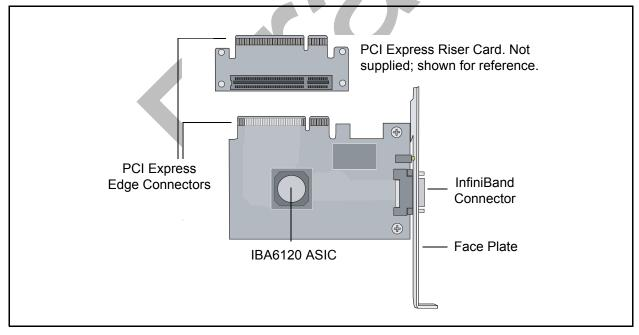
Figure 4-2. QLogic QLE7140 Card with Riser, Top View
